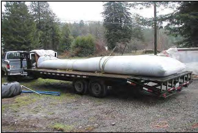
This AquaDam® has been used to convert a flatbed trailer into an instant water tank.
