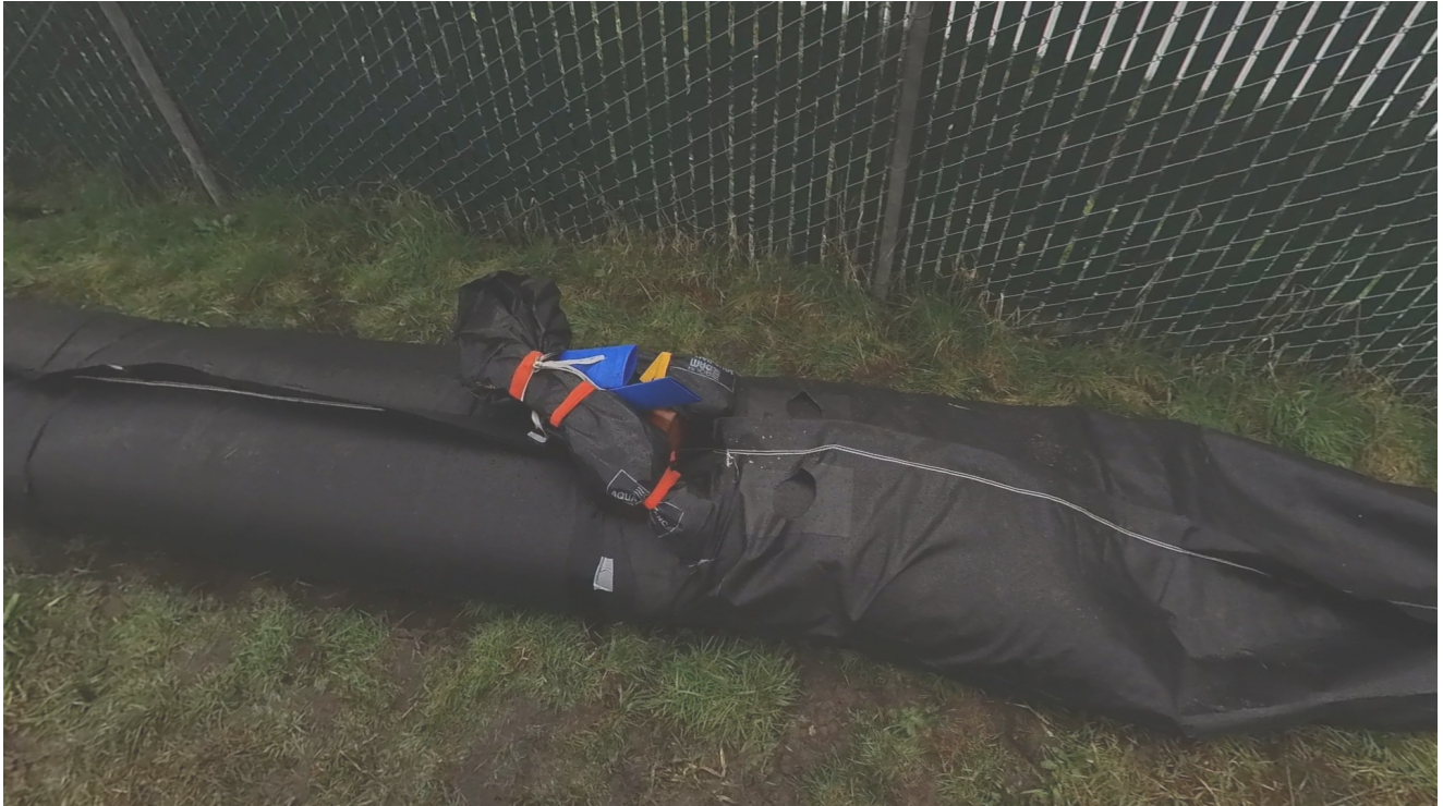
Image 6: AquaDams fill tube secured but leaning over and allowing water to spill out.
